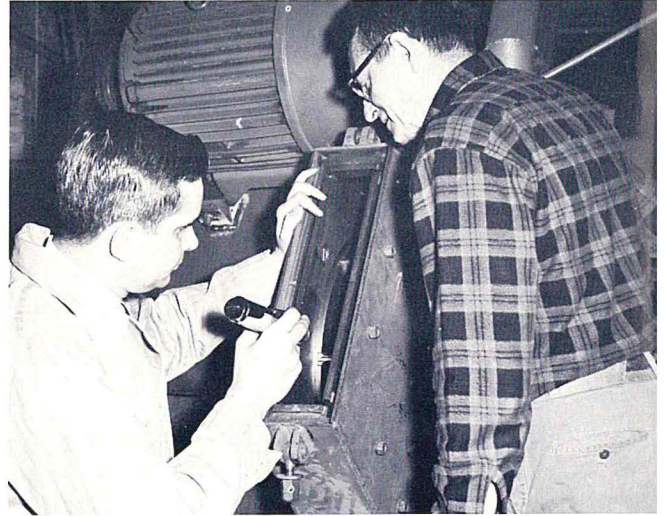
Wheelabrator field engineer checks the blast wheels — heart of every blast machine.
